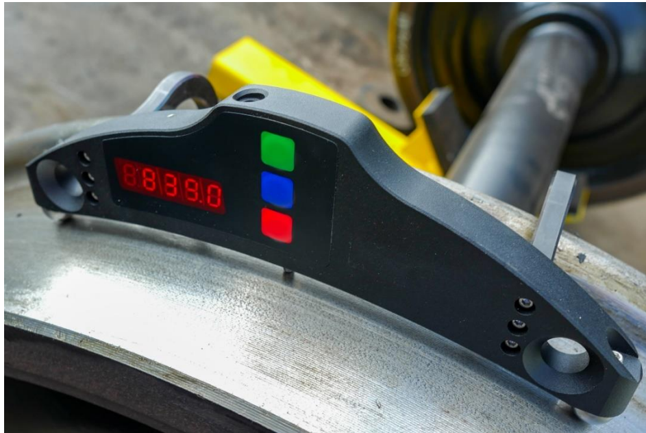
Fig. 1. Electronic wheel diameter measuring instrument ( https://www.ascorail.pl/en/electronic-wheel-diameter-measuring-instrument.html )
