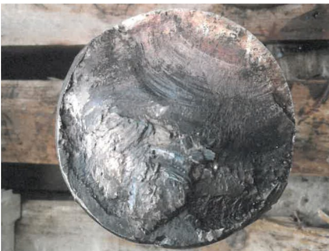
Fig. 8. Fatigue cracking surface of the axle of the freight wagon [5]
