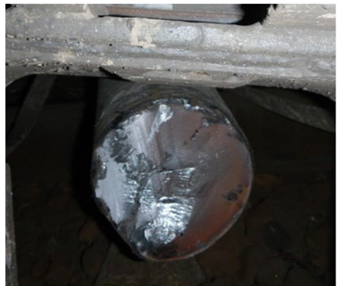
Fig. 5. Fatigue cracking surface of the axle of the freight wagon [4]
