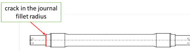
Fig. 7. The place of the axle fatigue crack
