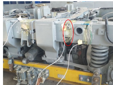
Fig. 7. Placement of strain gauges and their connection on the bogie frame of the transition type non-motor subway car of the model 81-714 Uz.
