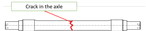
Fig. 4. The place of the axle fatigue crack
