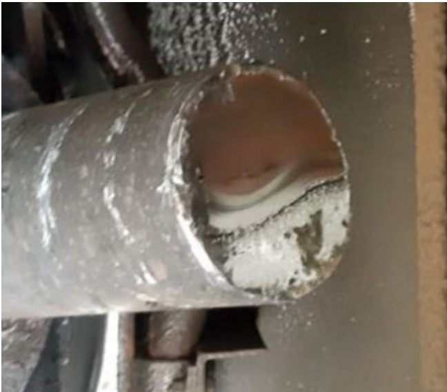
Fig. 6. Fatigue cracking surface of the axle of the freight wagon [4]
