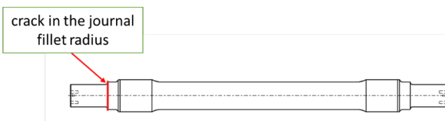
Fig. 7. The place of the axle fatigue crack
