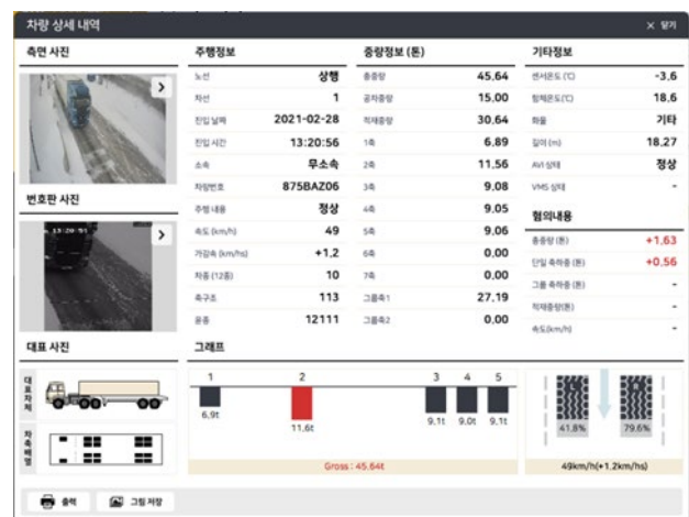
Figure 2. Talapker WIM data acquisition
