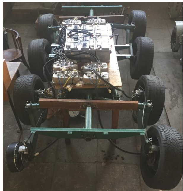
Fig.1. Experimental sample of vehicle with eight non-steering wheels.
